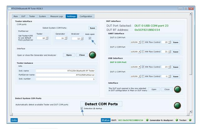
Check the **[Auto open]** option to automatically open the Generator and Analyzer COM ports when starting the RTX2254 application. Uncheck to disable auto open.
