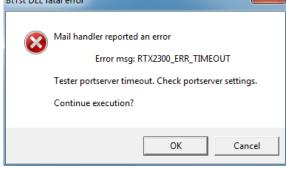
If the error pop-up looks like the following, then the RTX EAI Port Server are probably failing and you must configure it correctly.
