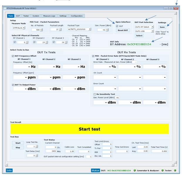
The RTX2254 Bluetooth RF tester is now configured and ready for testing.
