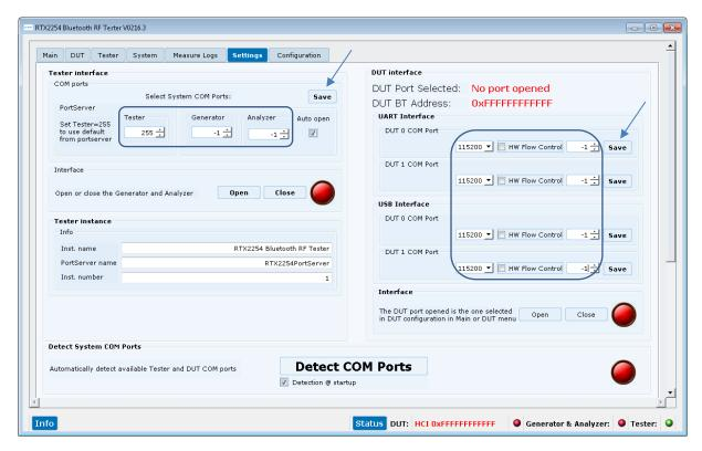
Enter the COM port number for the **[Tester interface]** and set the DUT configuration in the **[DUT Interface]** as required by your specific DUT.
