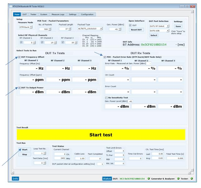
Make sure that the requested tests are enabled "DUT Frequency Offset", "DUT Tx Output Power" and "PER – Packet Error Rate".
