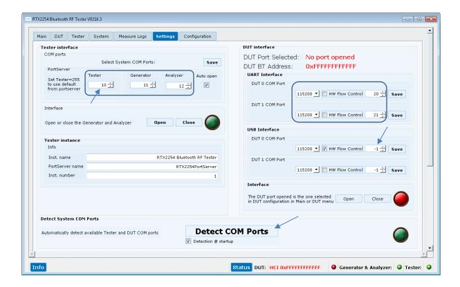
Click the [Detect COM Ports] to make a new COM port detection:
