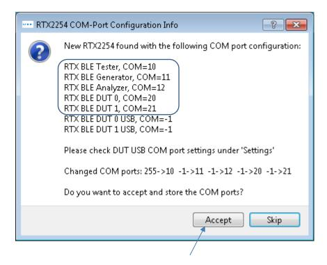
The RTX2254 application should find 4 COM ports for a RTX2254 single port version and 5 COM ports for a dual port version.
