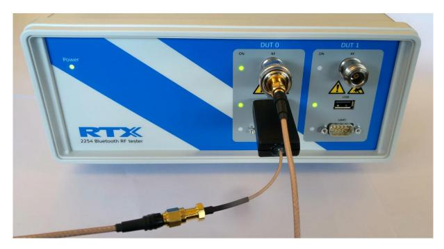
"Test DUT" is connected to DUTO RF and USB
