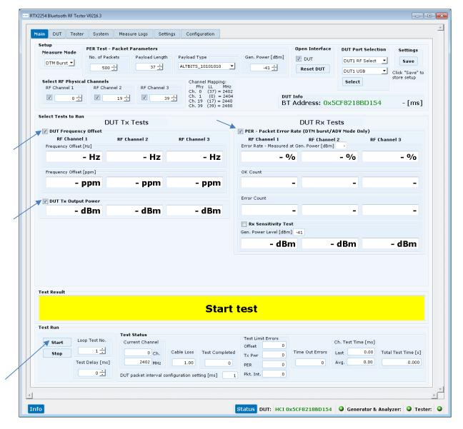
Make sure that the requested tests are enabled "DUT Frequency Offset", "DUT Tx Output Power" and "PER – Packet Error Rate".
