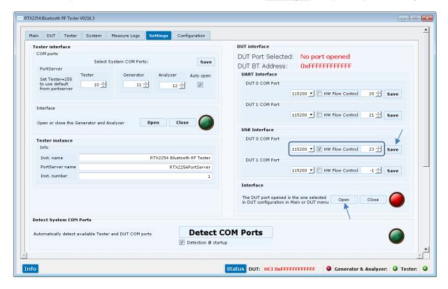
Set the DUT configuration (baud rate, HW flow control) as required by your specific DUT.
