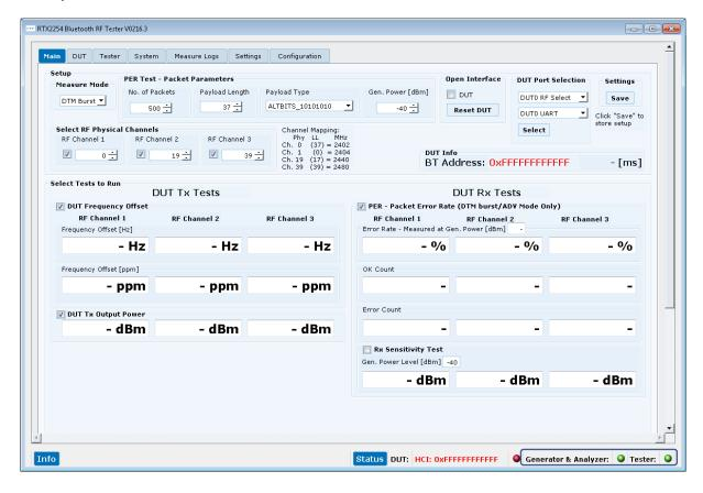
The interface status for the 3 internal instruments (Tester / Analyzer / Generator) should be green. The DUT has not been setup or opened and DUT status is red.
