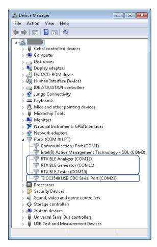
RTX2254 COM port 10,11,12 "Test DUT" on USB COM 23
