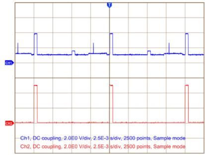
CH1: Online calibration, RTX2012 TX, FP TX. CH2: Timeslot for FP TX
