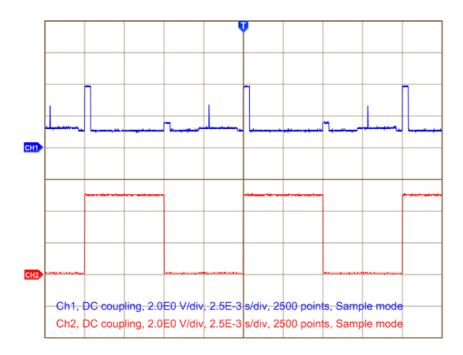
CH1: TX from device (FP), TX from RTX2012, online calibration CH2: Clock 100 synchronizing for RTX2012 TX
