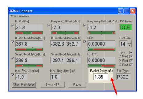
The measured Packet Delay could also be read out by sending the SCPI command **READ[:SCAL]:PACK:DEL?** (for more details please refer to the "Programming Reference"). Please note that this command will return three values – i.e. the actual packet delay and the minimum and maximum packet delay (all in  $\mu$ s).
