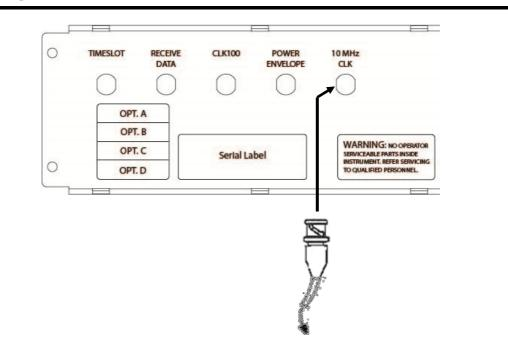
Connecting a cable to the BNC 10 MHz CLK Connector
