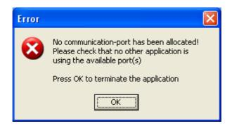
Please click **OK** and check all connections between the PC and tester along with the Power LED on the front panel. If the power LED is lit the tester should be operational, and hence, please check and/or replace the USB cable between the PC and the tester and try launching the application again.
