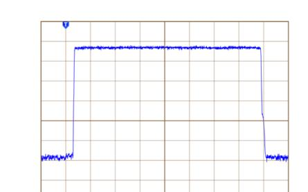
Ch1, DC coupling, 5.0E-1 V/div, 5.0E-5 s/div, 2500 points, Sample mode
