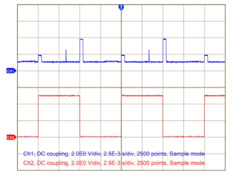
CH1: TX from device (PP), TX from RTX2012, online calibration CH2: Clock 100 synchronizing for RTX2012 TX
