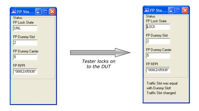
If the DUT has been set in test mode the RTX2012 tester can lock onto the device and the **FP Lock State** will change to LOCK when locked on to the DUT (see above). Please note that the Traffic Slot will be changed automatically if the Dummy Slot is the same as the defined Traffic Slot (as indicated in bottom of the FP Status window above).
