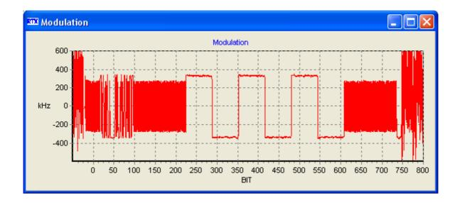
Please note that a higher number of bits are included than in the "normal" P32Z case. This is also the case with the NTP graph (see below). If the NTP graph does not match please check that you are using the correct power template.
