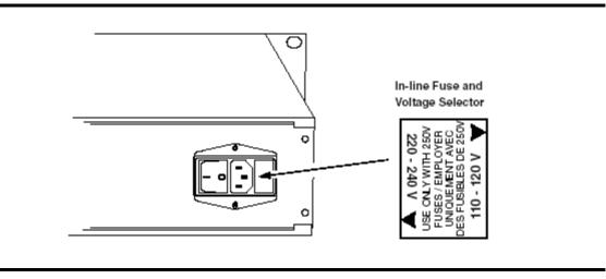
Check the operating voltage setting and fuse rating
