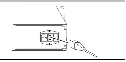
The tester is switched ON by pressing the Power Switch so that it is ON position (I).
