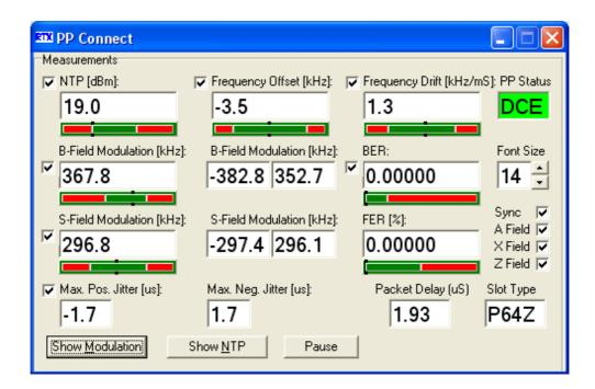
As a last step we can verify that a CAT-iq connection has been established by checking the **Slot Type** on the **PP Connect** window. As indicated above the slot type is P64Z (i.e. CAT-iq).
