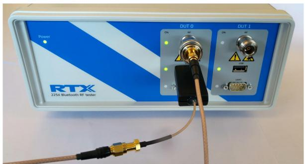
RTX2254 with "Test DUT" on USB
