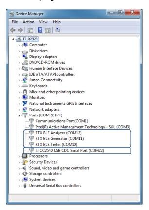
RTX2254 COM port 10,11,12 "Test DUT" on USB COM 22
