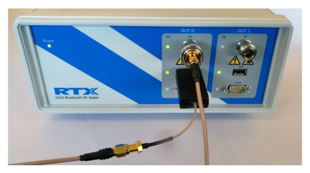
"Test DUT" is connected to DUT0 RF and USB
