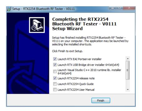
By default, 2 different drivers and optionally the development environment can be installed. The installer will present 32 bit (X86) or 64 bit (x64) drivers depending on the used PC's operating system.
