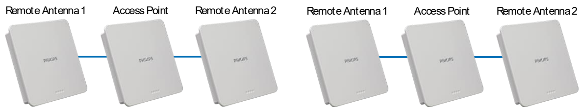
Figure 15: A Linear Access Point Deployment
