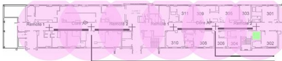
Figure 18: Linear Multiple Access Point Deployment
