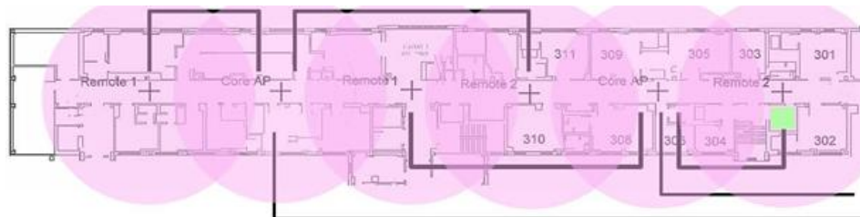
Figure 19: Interleaved Multiple Access Point Deployment
