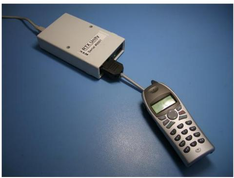
Figure 3. RTX Unity connected to SC14428 target.
