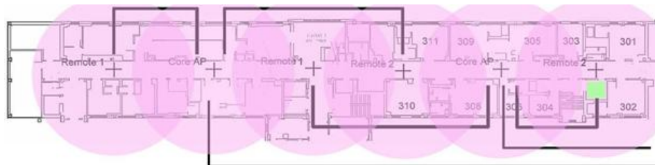
Figure 19: Interleaved Multiple Access Point Deployment
