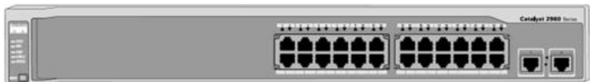
Figure 7: Power over Ethernet Switch
