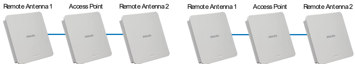
Figure 15: A Linear Access Point Deployment
