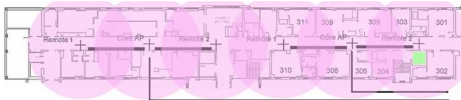
Figure 18: Linear Multiple Access Point Deployment
