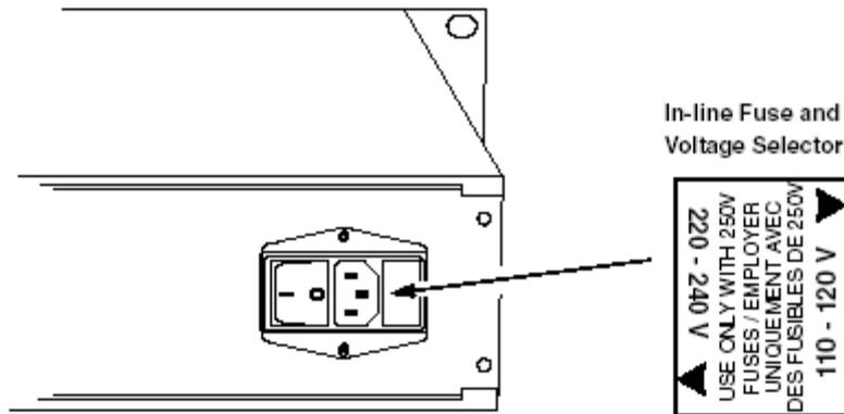
Select the required operating voltage by removing and replacing the fuse holder as shown below and ensure that the correct fuse is fitted.
