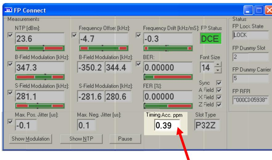
As indicated in the screen shot above the measured Timing Accuracy in ppm (parts per million) is 0.39.
