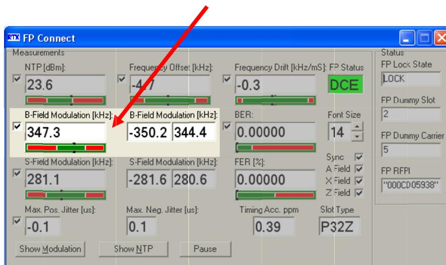
As indicated in the screen shot above the measured B-Field Modulation is 347.3 kHz.
