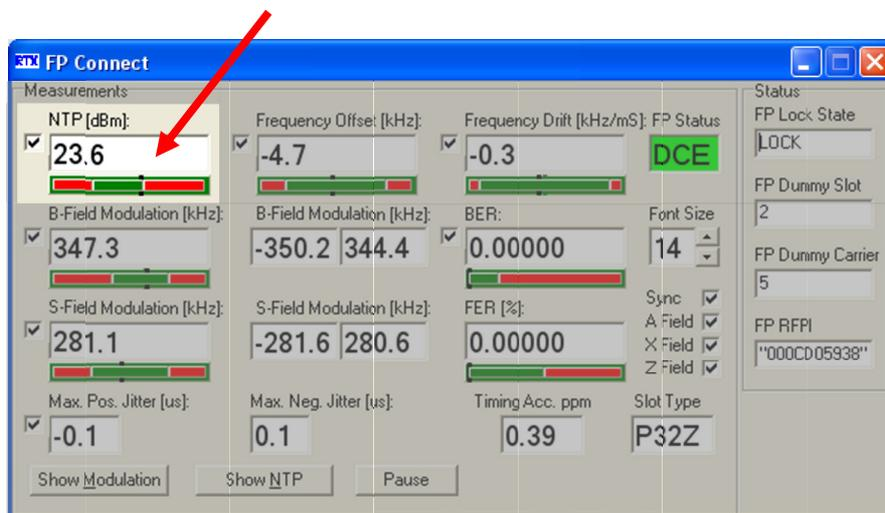
As indicated in the screen shot above the measured NTP power of the DUT is in this case 23.6 dBm. Please note that the measured NTP power value is within the limits specified in the **Setup FP** pane for NTP power (indicated by a green frame and a value indicator within the green area).
