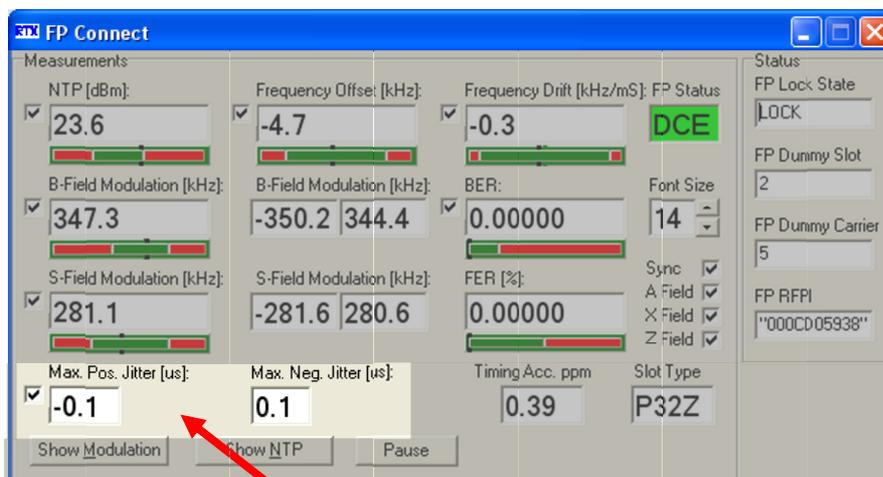
As indicated in the screen shot above the measured maximum positive jitter is  $-0.1 \mu\text{s}$  and maximum negative jitter is  $0.1 \mu\text{s}$ .
