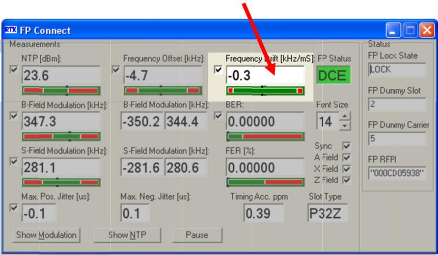
As indicated in the screen shot above the measured Frequency Drift is -0.3 kHz/mS (which is within the limits defined for this parameter). Please note here that the unit is set to kHz/mS – alternatively this could be kHz/slot.
