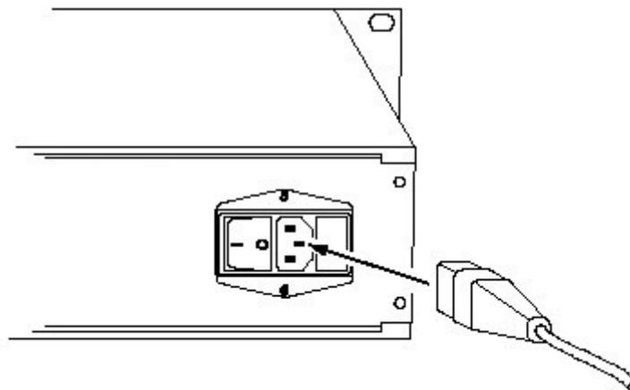
The tester is switched ON by pressing the Power Switch so that it is ON position (I).
