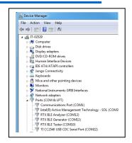
The RTX2254 has 3 communication interfaces: [Tester], [Generator] and [Analyzer].
