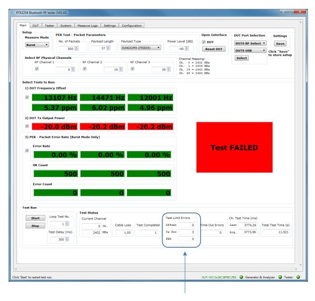
All Tx power tests are outside the test limits and failed
