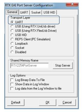
Setup the COM-ports for [Generator] and [Analyzer].
